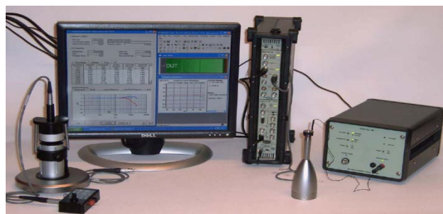
Фиг.5 Калибриране - Phase Response Comparison Calibration
