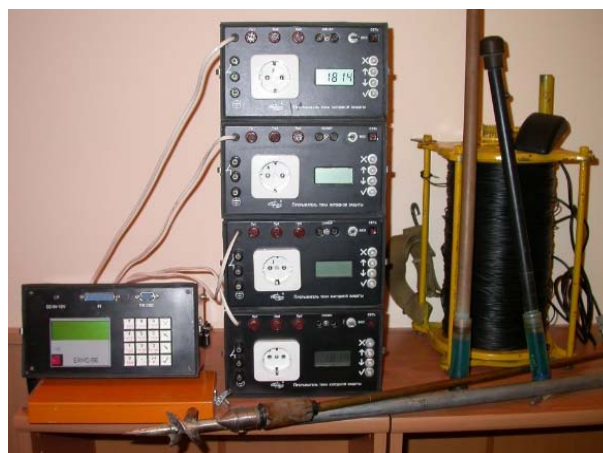
Fig. 6. The System Corrosion Monitoring of Pipelines
